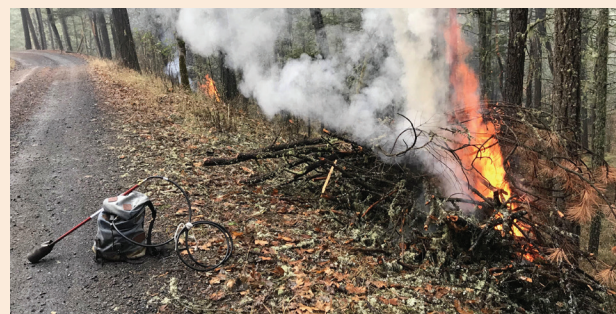
A propane torch is used to set fire to slash piles and conduct prescribed burns.
